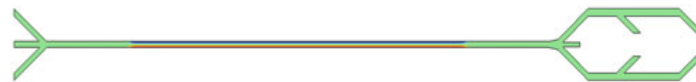
Microscale Acoustofluidics, Fig. 4 Acoustic pressure distribution in the channel because of piezoelectric excitation on the wall
