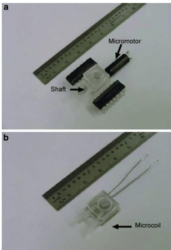
**Magnetic Pumps, Fig. 3** Test and measurement setup for two micropumps of different driving mechanisms: (a) permanent magnet with a small DC motor; (b) integrated coil (Reprinted from [5] with permission from Dr. Ziaie)
