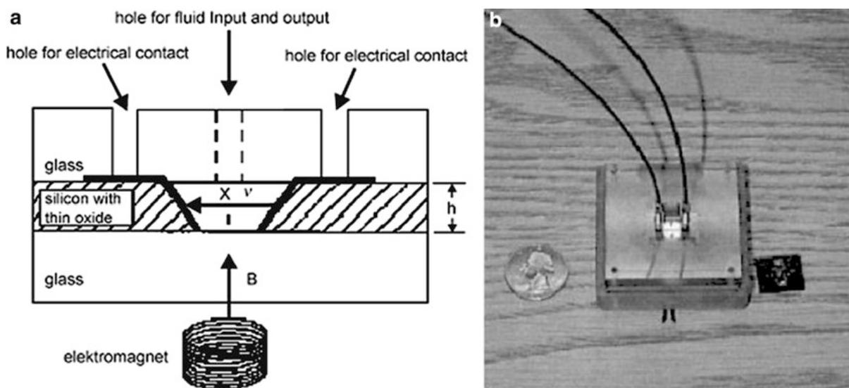
**Magnetic Pumps, Fig. 5** (a) Cross section of AC MHD and (b) photograph of microsystem of (Reprinted from [9] with permission from Dr. Lee)
