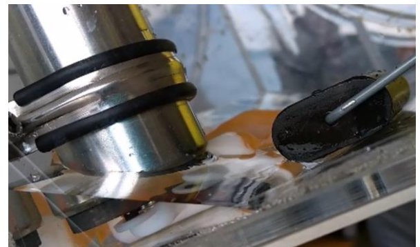
Fig 12. Trapped fluid of case 1 with 25 degree tilting condition.
