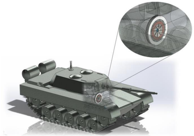
Figure 2. The location of electro-mechanical clutch in the military system[2]
