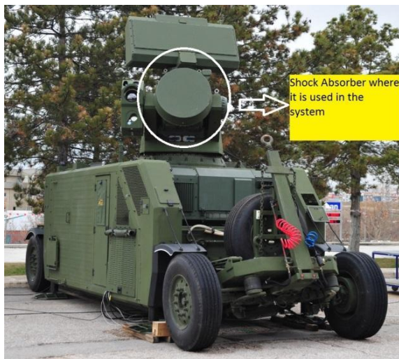
Figure 1 -The place of shock absorber where it is used in the radar system [1]
