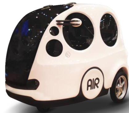
Figure 2. Usage of compressed air engine in a small vehicle [1]
