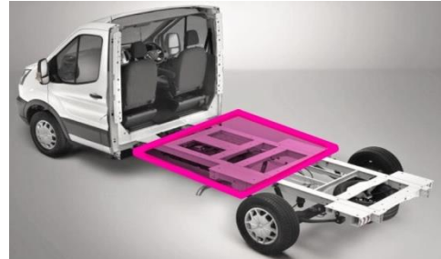
Figure 2: Position of the Battery Pack in Accordance With the Vehicle's Main Chassis [2].
