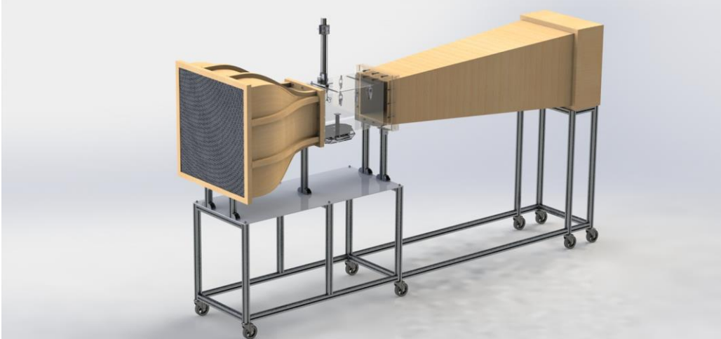
Figure 4: Overall CAD Design of Wind Tunnel
