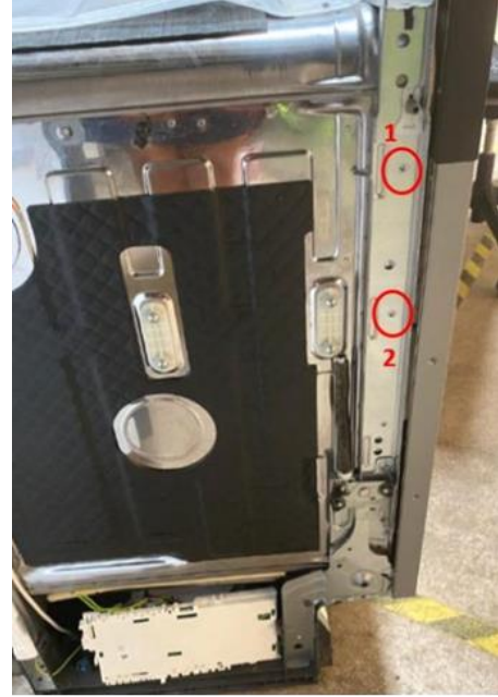
Figure 2: Clinching points on an Arçelik dishwasher .
